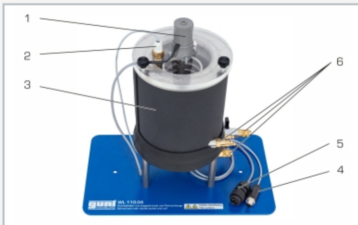
1 stirring machine, 2 temperature sensor, 3 stirred tank, 4 temperature sensor connection, 5 stirring machine connection, 6 water connection jacket, stirred tank, coiled tube water connection
